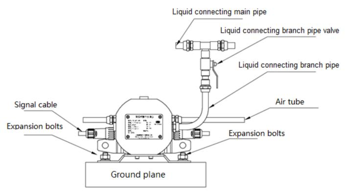
Flat mounted: Screw-fixed type diagram
