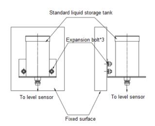
Standard liquid storage tank installation diagram
